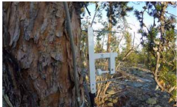
Dendrometer Installed on a jack pine.
