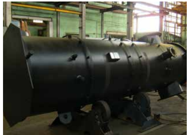
New Heat Recovery Unit in the factory.
