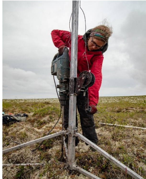
Western Arctic Research Centre Permafrost Specialist, Alice Wilson, drills permafrost cores to gather data to support climate change research
