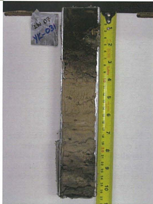
Figure A-1B: Photograph of the Site 31 core at Giant after being split longitudinally, thawed and air-dried. Sample shows high organic content at the surface, followed by the presence of clay rich material at depth.
