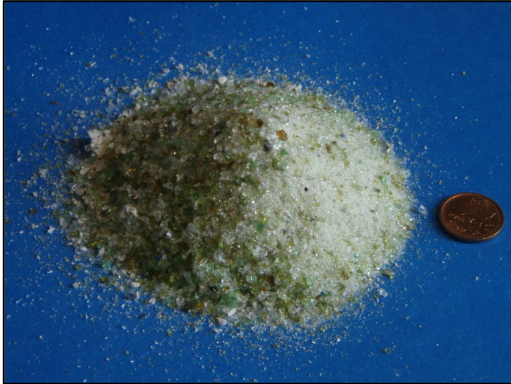
NWT glass after being processed in Airdrie. The “sand” will be spun into glass fibres and will eventually become fibreglass insulation.
