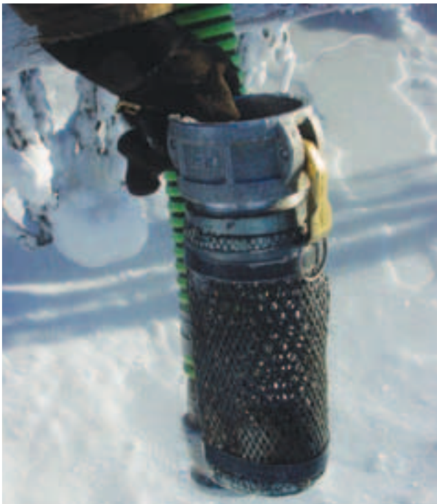
FIGURE 13. Intake screens for water withdrawal should meet Fisheries and Oceans Canada's Freshwater Intake End-of-Pipe Fish Screen Guidelines.
