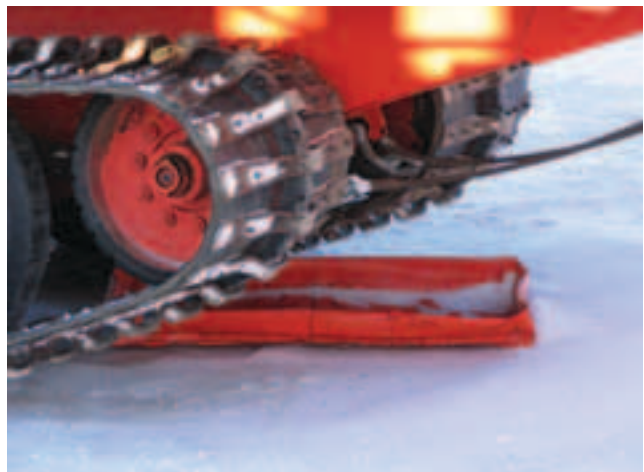
FIGURE 37. Drip trays should be placed under parked equipment to catch unexpected drips or spills.
