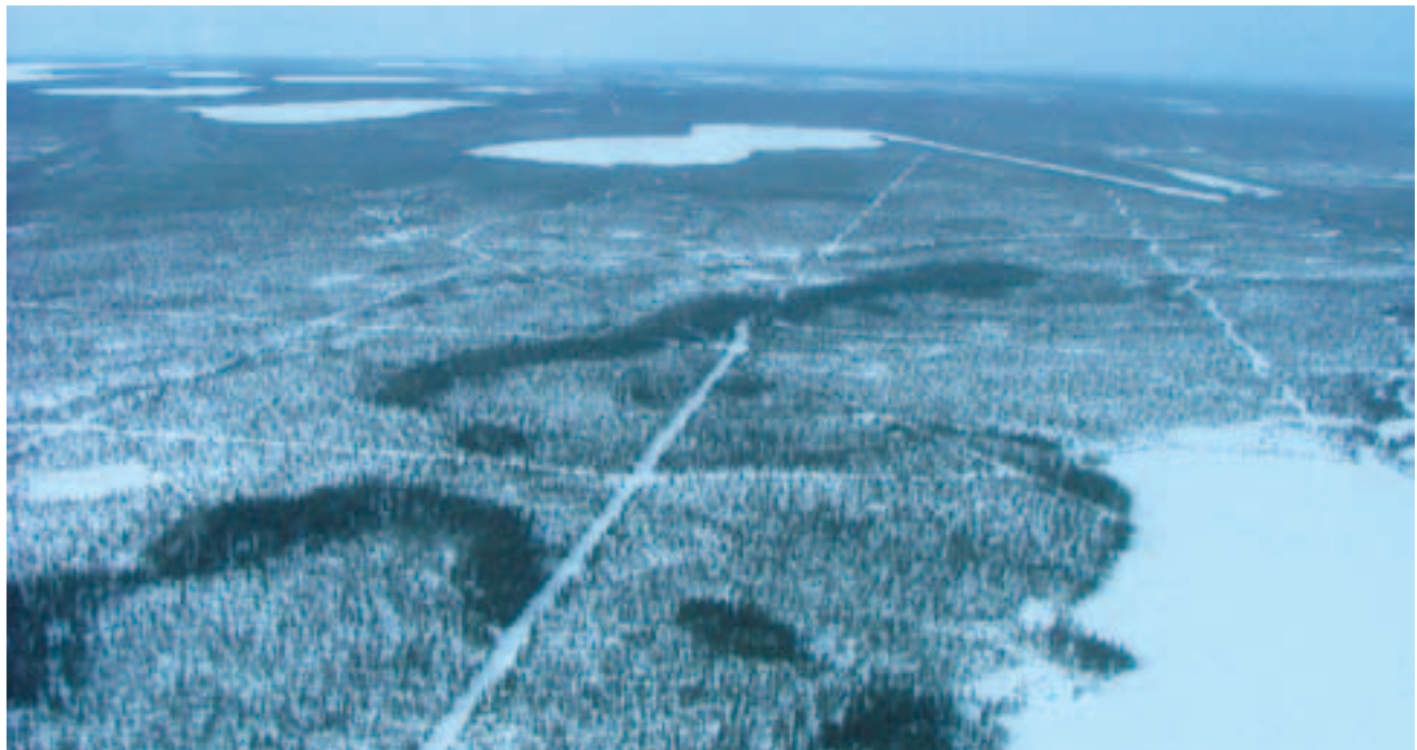
FIGURE 8. Use existing disturbances and natural openings, where appropriate, to minimize the project’s footprint. Some of these existing cutlines could be used for access to a new seismic program site.
