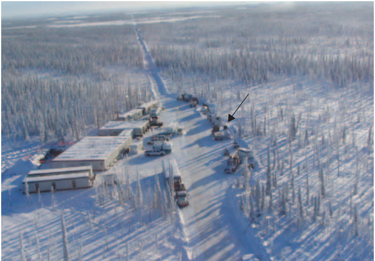
FIGURE 34. Minimal fuel is stored at this mobile camp in a double-walled tank, indicated by the arrow.
