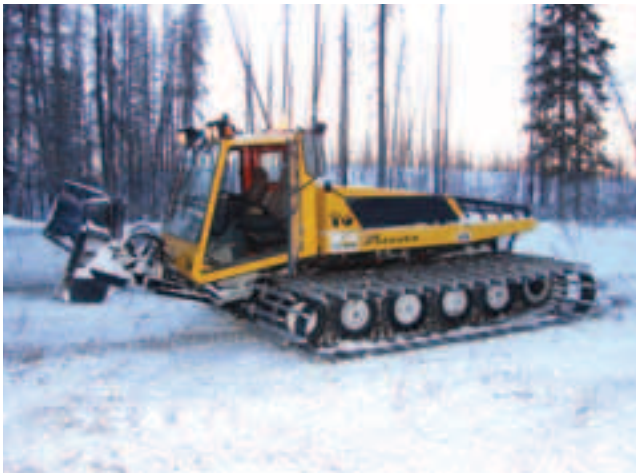
FIGURE 20. Use of low ground pressure equipment is recommended in tundra terrain.
