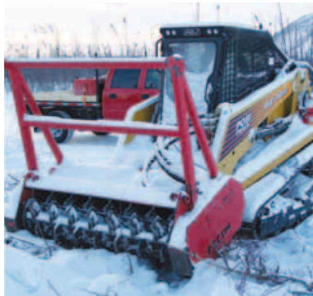
FIGURE 29. A mulcher used for brush disposal.
