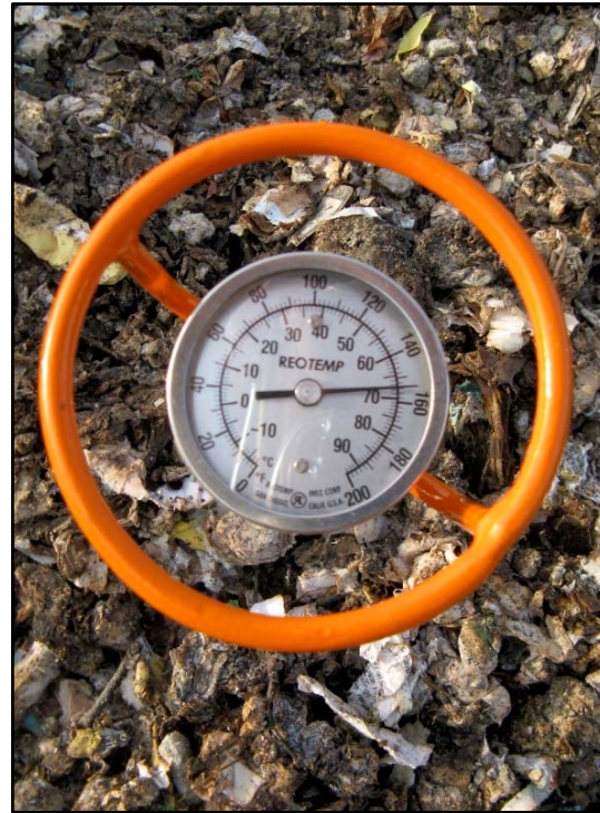
Composting windrow reaching 67°C
