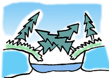
Melting permafrost can create cavities ...
