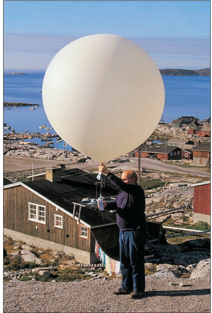
This Greenlandic meteorologist is releasing a weather balloon so that he can observe the air currents. From his observations, he will be able to make some predictions about the weather.
