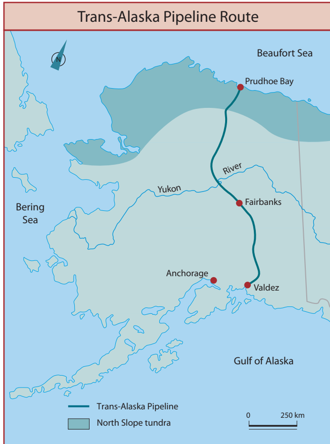
The Trans-Alaska Pipeline extends 1300 kilometres, from Prudhoe Bay to Valdez. It now carries an average of 720,000 barrels of oil a day.
