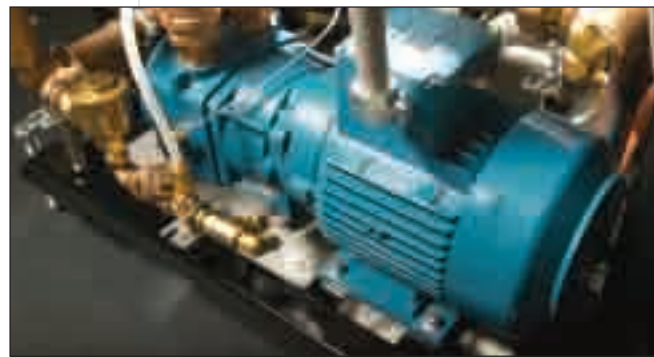
Two-stage vacuum pump reduces water consumption and provides quick, quiet, consistent chamber evacuation
