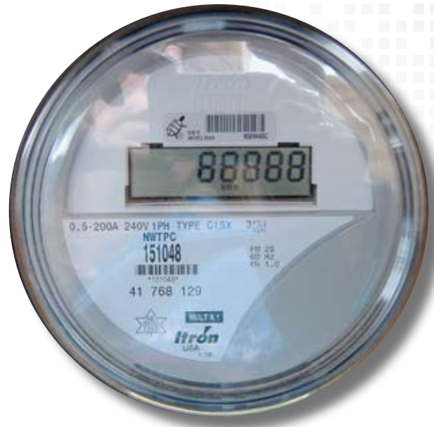
Electronic meters are read by computer, eliminating the need for a monthly visit to every home.
