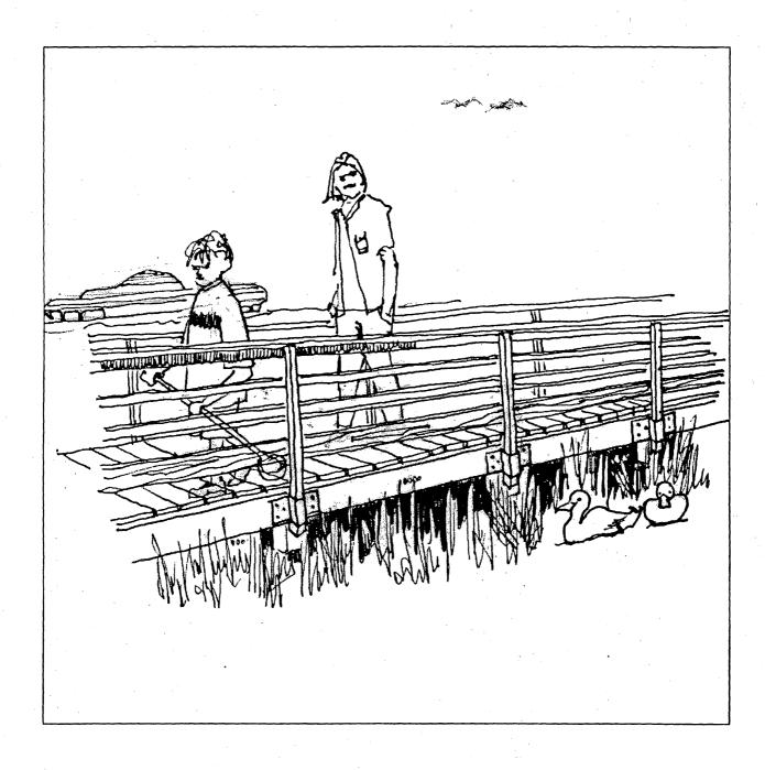
boardwalk above ground level. A strategy, similar to that used to attached decking to some marine pilings, would allow the boardwalk to be adjusted up or down to accommodate changes in the surface levels caused by permafrost heave or settling.
