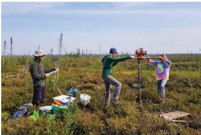
Sahtu research team using SIPRE drill for taking frozen soil samples. Photo by A. Sniderhan
