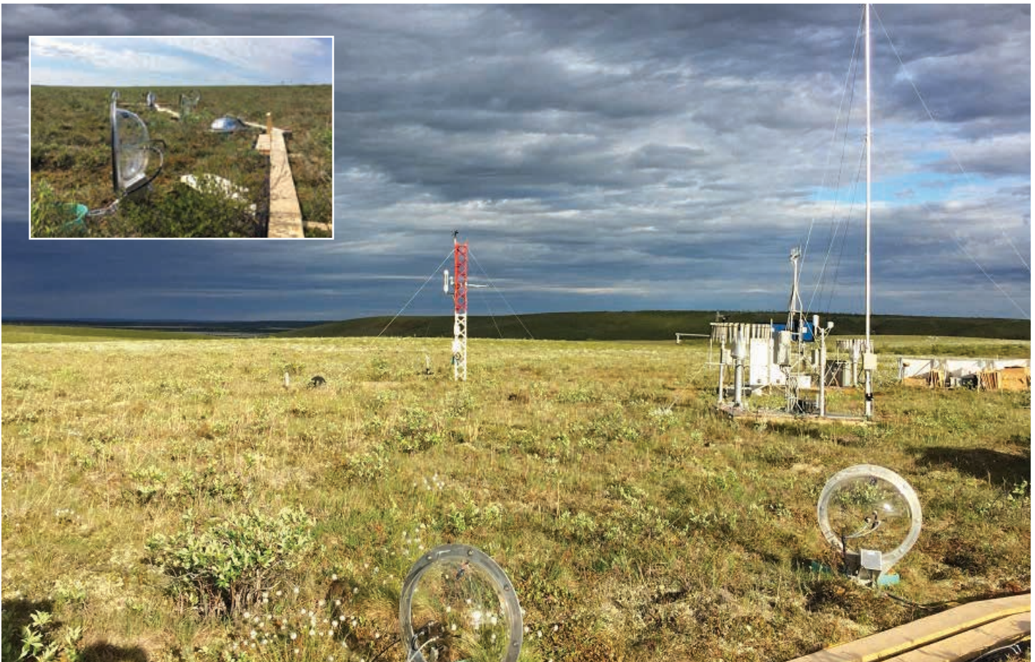
Eddy covariance tower and automated chambers measuring carbon and water fluxes at Trail Valley Creek Research Station, June 2019. Photo credit: C. Voigt Inset photo: Automated chamber set-up with transparent and dark chambers at Trail Valley Creek Research Station, June 2019. Photo credit: C. Voigt
