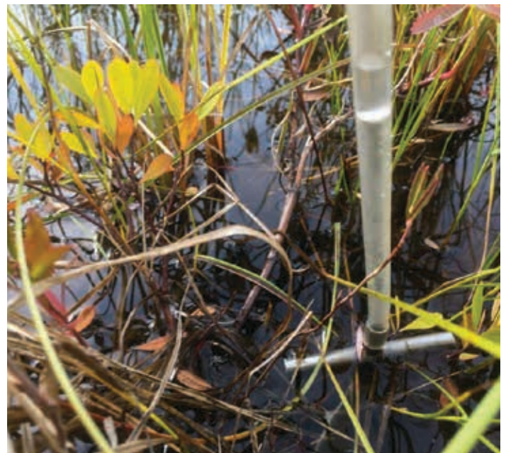
Photo of groundwater sampling procedure at a spring. The portable sampling instrument is installed to a depth of about 1 m below the ground surface. Water at this depth is under artesian pressure, and so it rises in the tube above the height of the ponded water at the surface. Water is collected from this depth to analyze for water quality and isotopes.
