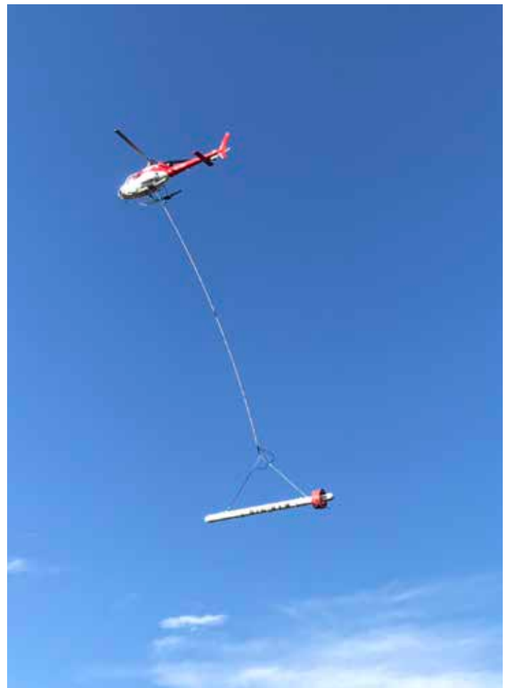
The Resolve6 Airborne Electromagnetic system (AEM) in operation. Photo credit: Xcalibur Multiphysics
