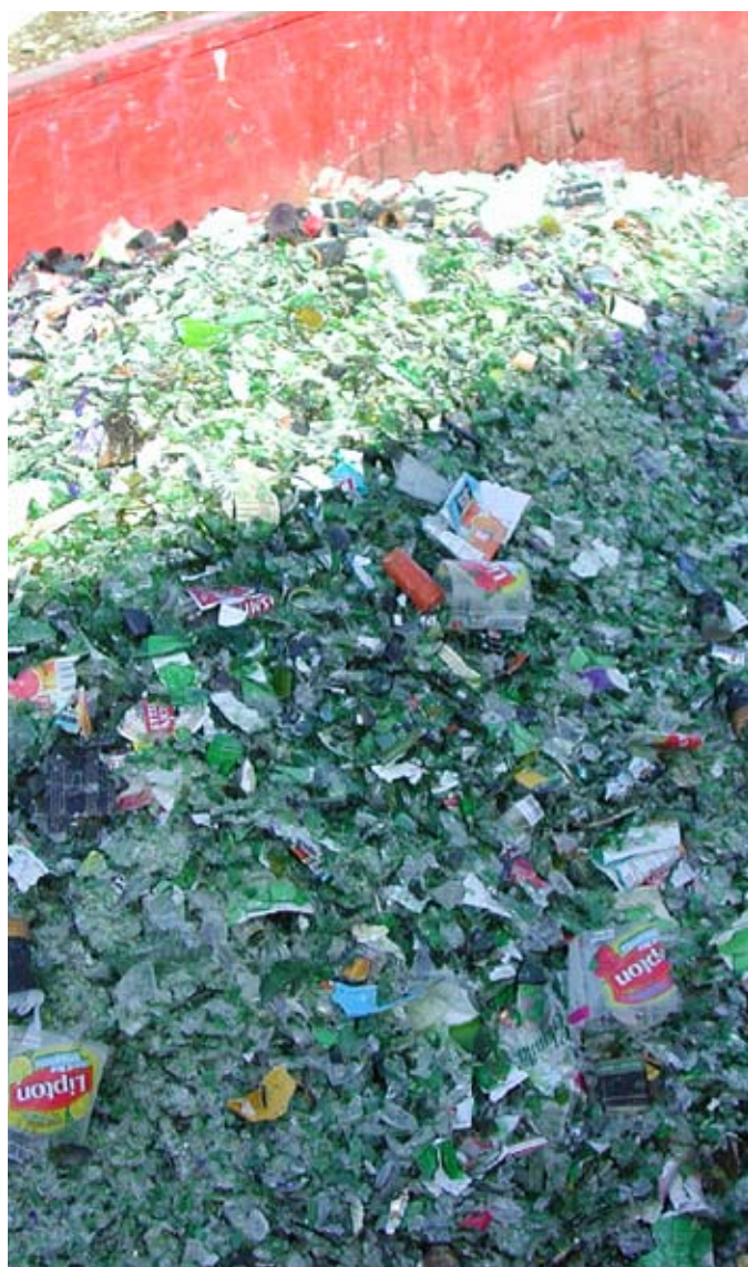
Although glass has little market value, it has found a home as backfill in new construction in Yellowknife and Hay River.
