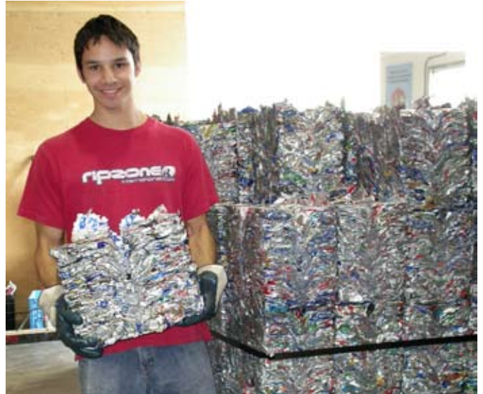
Aluminum cans are sent to a regional processing centre, like this one in Yellowknife, where they are crushed into briquettes. Each briquette weighs 12.25 kg (27 lbs.) and contains about 800 cans. They are sent south for recycling and then are made into new cans and other products.
