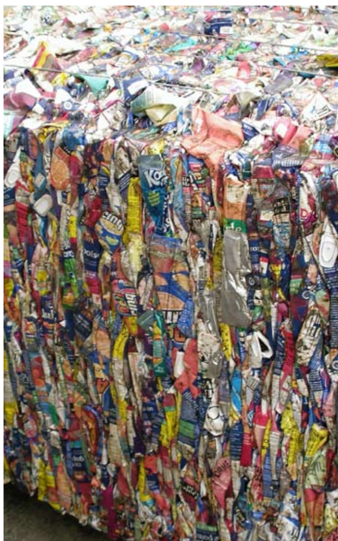
Multi-material containers such as Tetra-Paks, juice boxes and gable top containers must go through a process called hydropulping to separate the different components of the containers in the recycling process. These containers are made into cardboard, napkins, and plastic wood.
