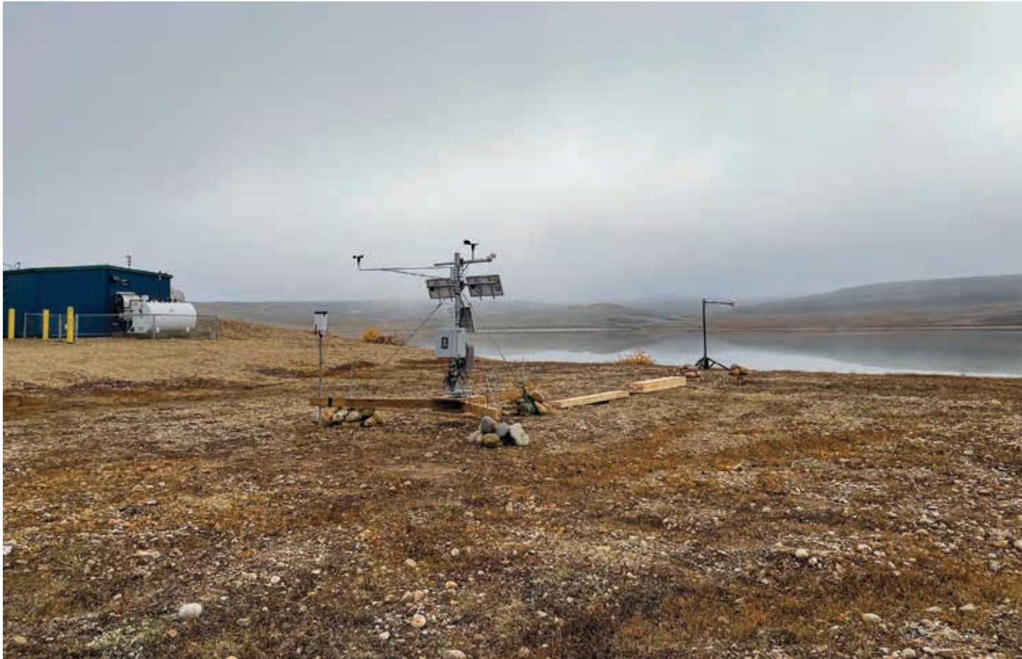
Equipment has been set up in Paulatuk to gather wind and solar data in the High Arctic community.
