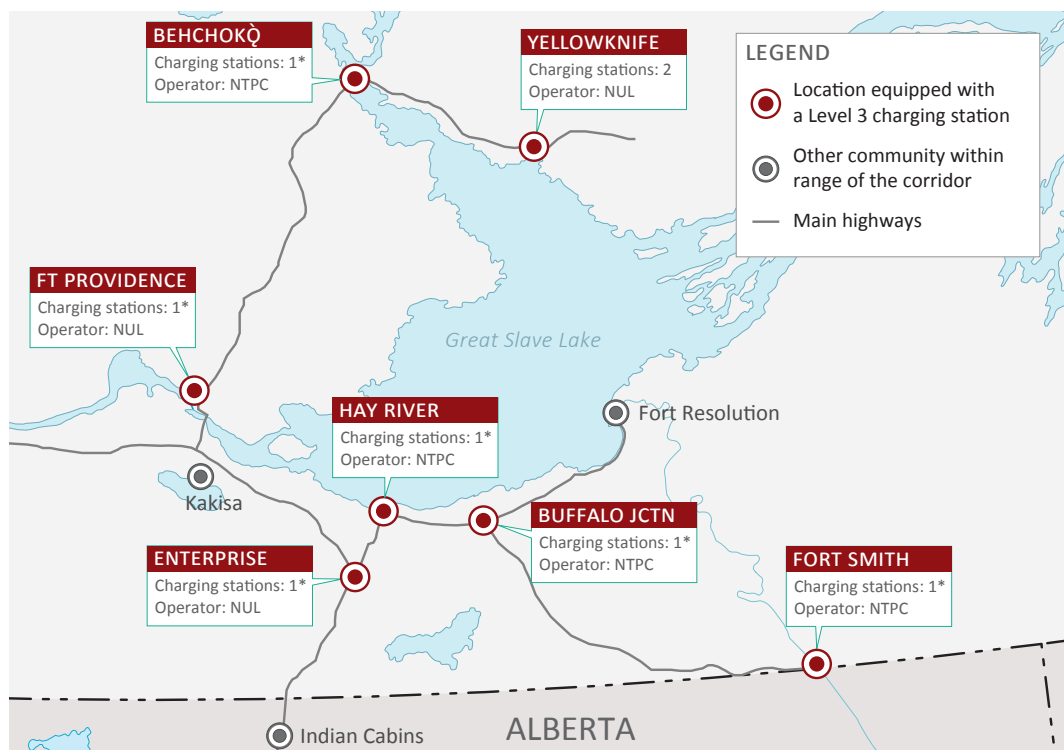
Figure 9 shows the locations of the Level 3 chargers forming a zero-emissions corridor around Great Slave Lake. * Location equipped with an additional Level 2 charging station for redundancy purposes.
