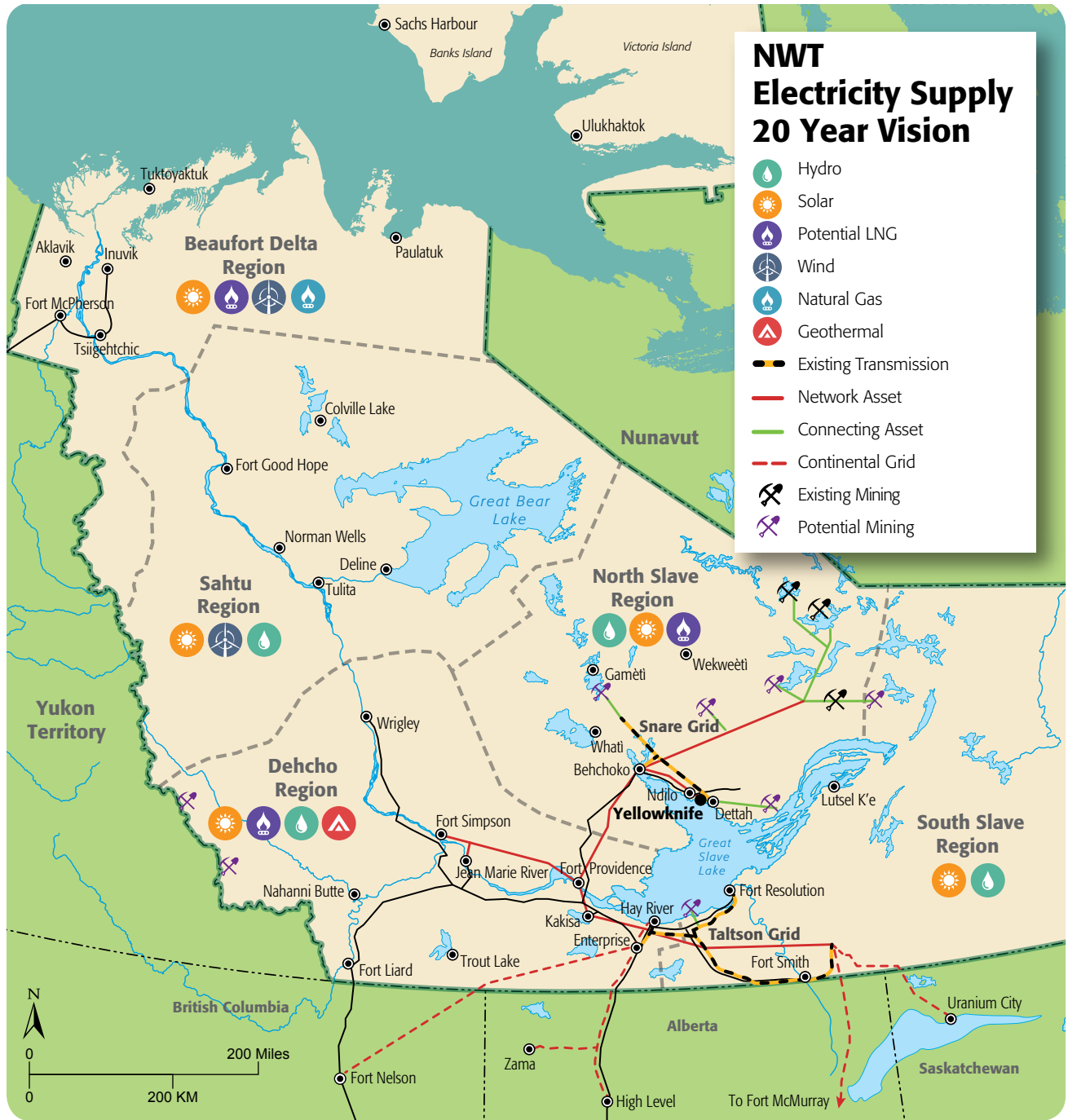
Figure 1 – NWT Electricity Supply 20 Year Vision
