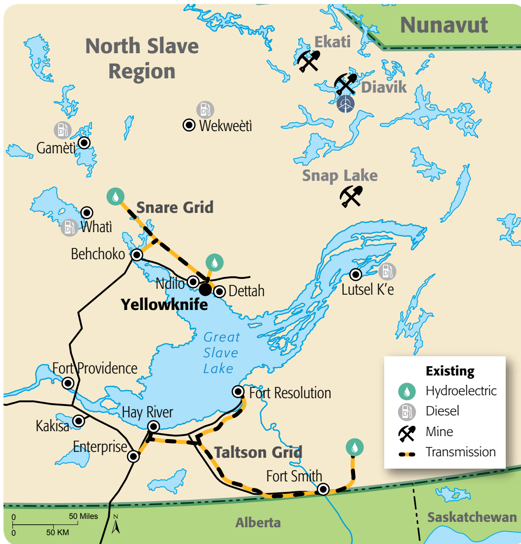
Figure 7 – North Slave Region Communities and Electrical Infrastructure
