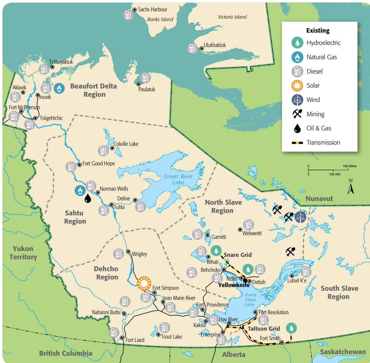
Figure 2 – Existing Electrical Infrastructure of the NWT
