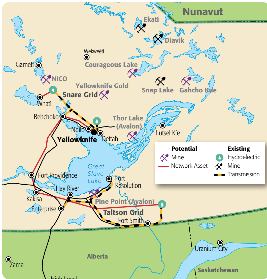
Figure 16 – West Slave Transmission Line (WSTL)
