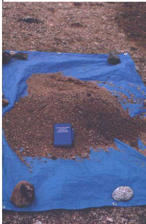
Photo 4: Sample taken from a borehole. The sample is coned and quartered before being sealed for transport.
